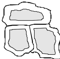
Figure 4. A schematic description of the GB regions. The gray areas present homogeneous perovskite manganites. The white areas are boundary-regions between grains, where structural distortions, stoichiometric deviations, crystal-orientation-mismatches, oxygen deficiencies, strains, and other defects are supposed to exist.
