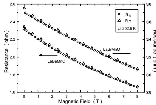
Figure 1. Field dependence of the ohmic resistance of  $\text{La}_{0.67}\text{Sr}_{0.33}\text{MnO}_3$  and  $\text{La}_{0.67}\text{Ba}_{0.33}\text{MnO}_3$  thin samples at 292.5 K. The circles and triangles represent the longitudinal ( $\mathbf{H}/\mathbf{J}$ ) and transverse ( $\mathbf{H}$  oriented in the sample plane, perpendicular to  $\mathbf{J}$ ) resistance  $R_{//}$  and  $R_T$ , respectively. There is a pronounced drop of  $R_{//}$  but not of  $R_T$  at low field.
