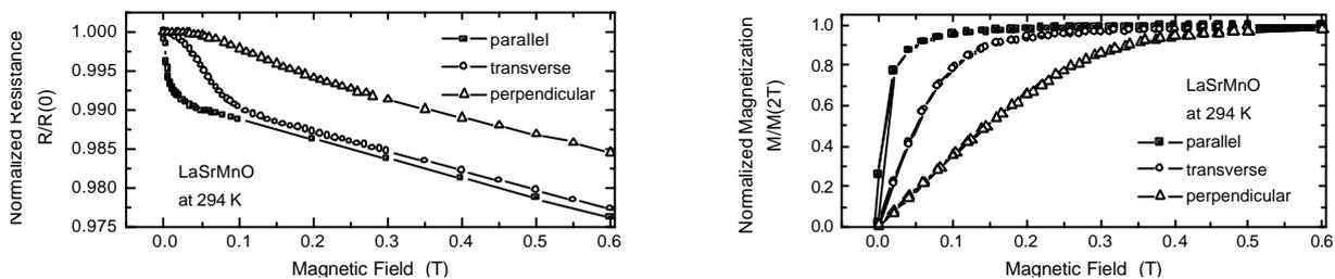
Figure 3. A comparison between the saturation fields  $H_s$  of magnetoresistance and magnetization for  $\text{La}_{0.67}\text{Sr}_{0.33}\text{MnO}_3$  stripes at room temperature and for different orientations of fields.
