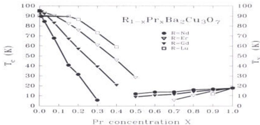
Fig.2.  $T_c$  and  $T_N$  vs  $x$  for  $(\text{R}_{1-x}\text{Pr}_x)\text{Ba}_2\text{Cu}_3\text{O}_7$  systems ( $\text{R}=\text{Nd}, \text{Gd}, \text{Er}, \text{and Lu}$ ).
