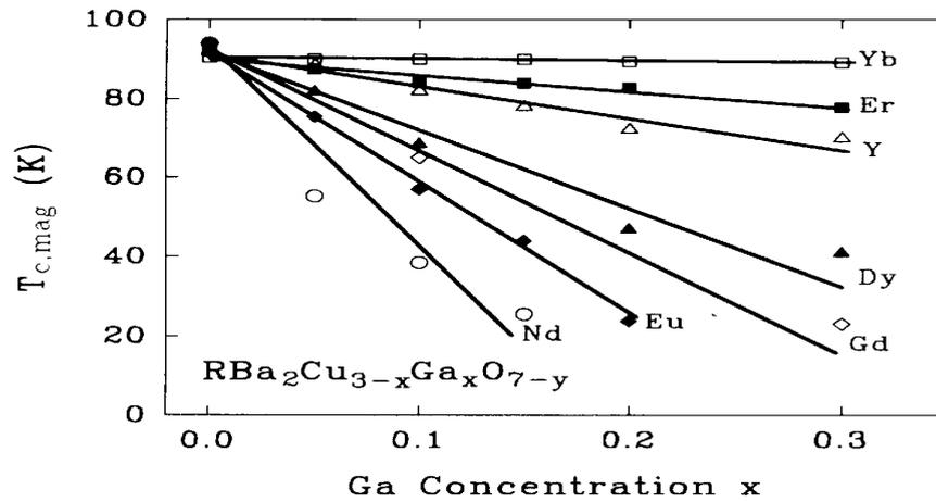
Fig.3.  $T_{c,mag}$  as a function of Ga concentration for  $\text{R}\text{Ba}_2\text{Cu}_{3-x}\text{Ga}_x\text{O}_{7-y}$  systems (R=Yb, Er, Y, Dy, Gd, Eu and Nd).
