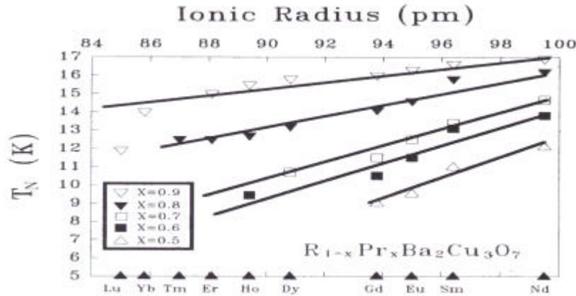
Fig.1.  $T_N$  vs ionic radius of R in  $(\text{R}_{1-x}\text{Pr}_x)\text{Ba}_2\text{Cu}_3\text{O}_7$  systems.
